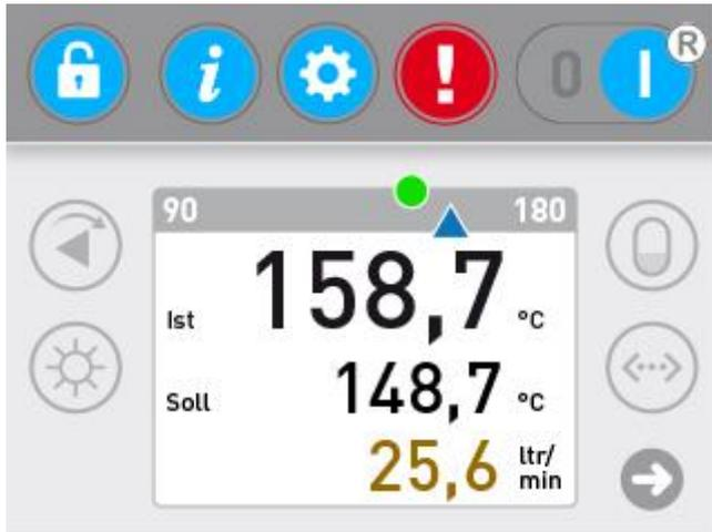
The SBC-T is equipped with a 3.5" touch screen. Operation is exclusively screen-based.
