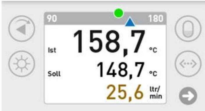
The actual temperature is the temperature that is included for the control. In the delivery condition, this is the temperature of the regular control sensor. You can configure the parameters to define that an external sensor is used for control instead.
